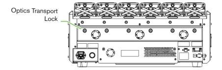
To engage the optics transport lock: use a size 4 Allen key to push the lock in and turn clockwise one quarter turn.
