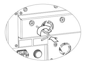
To disengage the optics transport lock: use a size 4 Allen key to turn counterclockwise one quarter turn.
