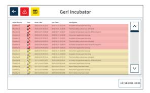
The alarms and warnings history screen displays a brief description of the alarm or warning, and where relevant, a start and end time for when the alarm or warning occurred.
