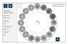
NOTE: If Geri has not detected the correct empty wells, tap on the correct empty wells and then tap the empty well icon in the top right corner. Perform this prior to tapping the record icon.
