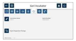
When two or more Geri instruments are being used, it is possible to assign each instrument an individual name to help distinguish between them.
