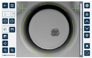
2. Use the arrow icons ^ v a v to adjust the camera focus as required.
