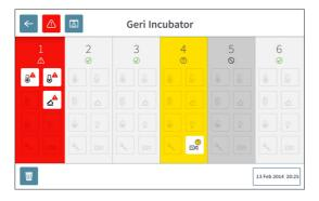
When an alarm or warning is activated, tap the alarm icon . The active alarm or warning is highlighted and the corresponding chamber will be highlighted red for an alarm or yellow for a warning. The specific alarm or warning is also highlighted.
