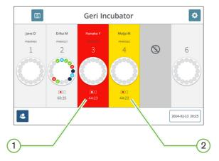
The corresponding chamber lid screen will also highlight the activated alarm or warning.
